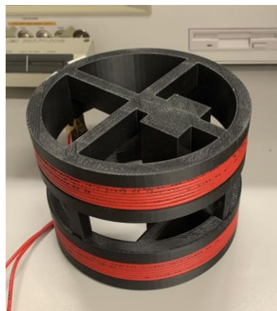
Figure 22: Helmholtz coils developed to fit inside the mu-metal chamber.
