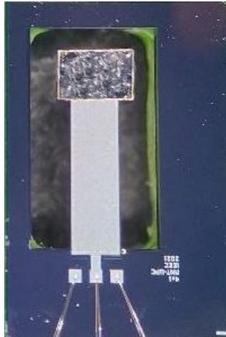
Figure 12: MEMS cantilever with mu foil tape attached.
