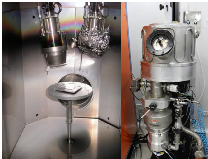
Figure 25: Sputtering (left) and evaporation (right) chambers
