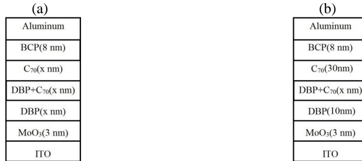
Figure 4. (a) Device structure for intrinsic layer optimization. (b) The structure used to fabricate PIN-junction cells
