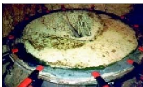
Figura 3.3 – Sofre incrustat a les parets internes del biodigestor [8]
