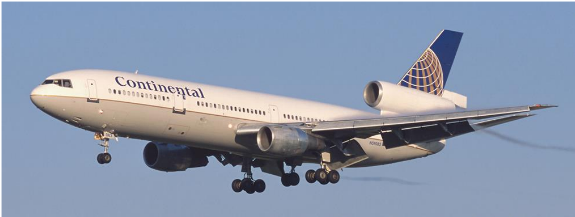
Figure 11: McDonnell Douglas DC-10-30 with two engines under wings and a central one in tail [Source: United Airlines].
