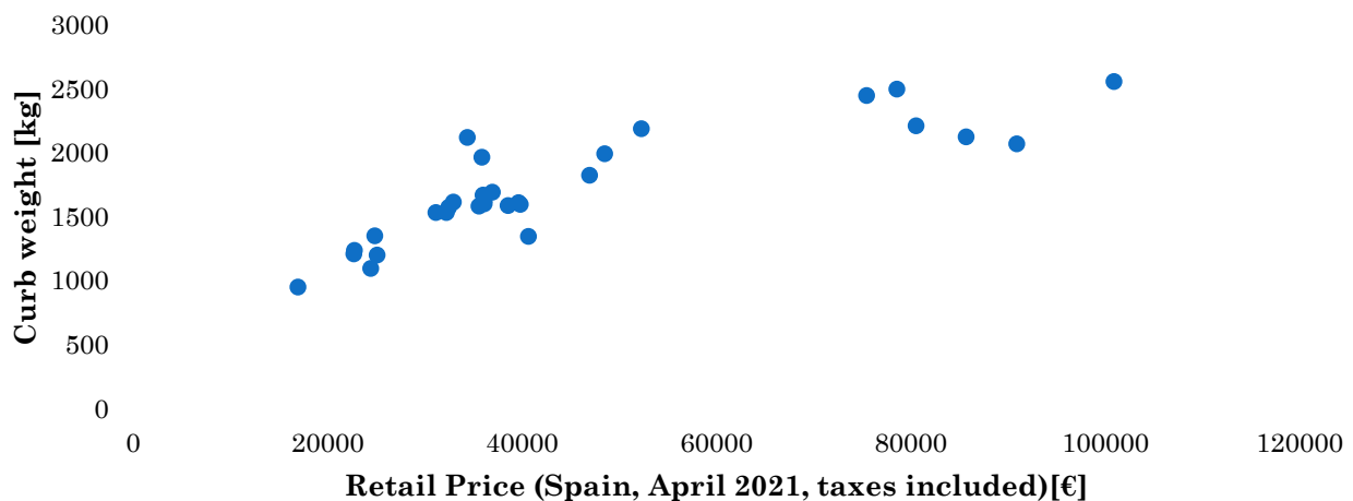
Figure 30 BEV Curb weight vs. price. Sources: (EVSpecs, 2020) (EVdatabase, 2020), (coches.com). Data in Appendix Table B-3 and B-4.
