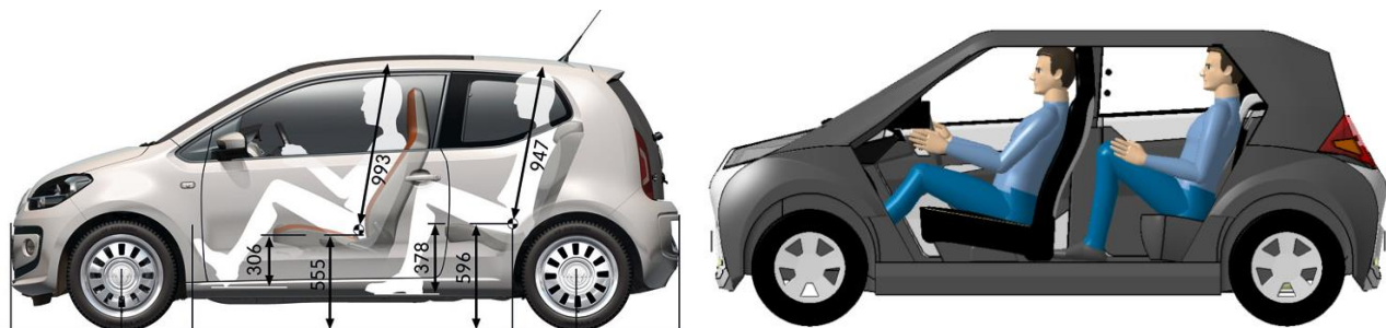
Figure 31 Interior space comparison. (Models not to scale between each other). Source: (CARICOS), own elaboration.
