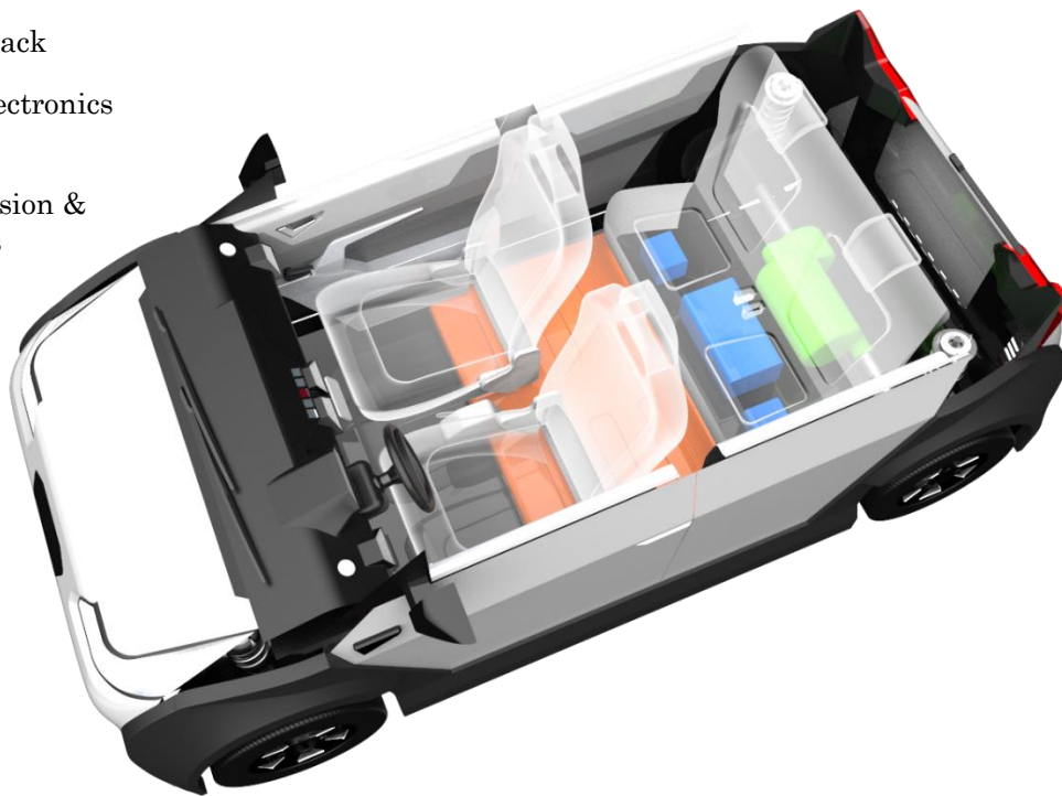
Figure 40. Powertrain components distribution. Source: own elaboration.
