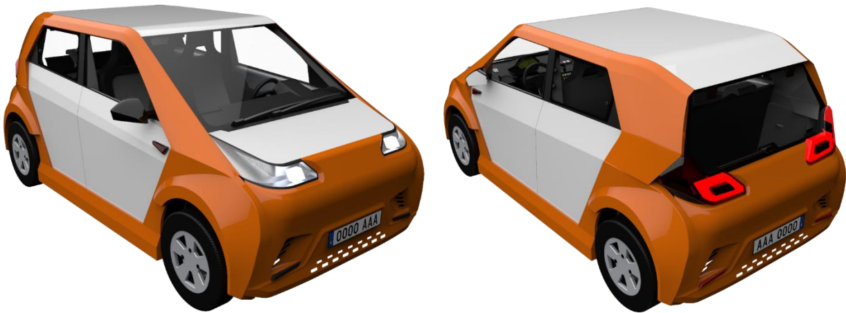
Figure 53. Plastic bodywork panels (orange). Source: own elaboration.
