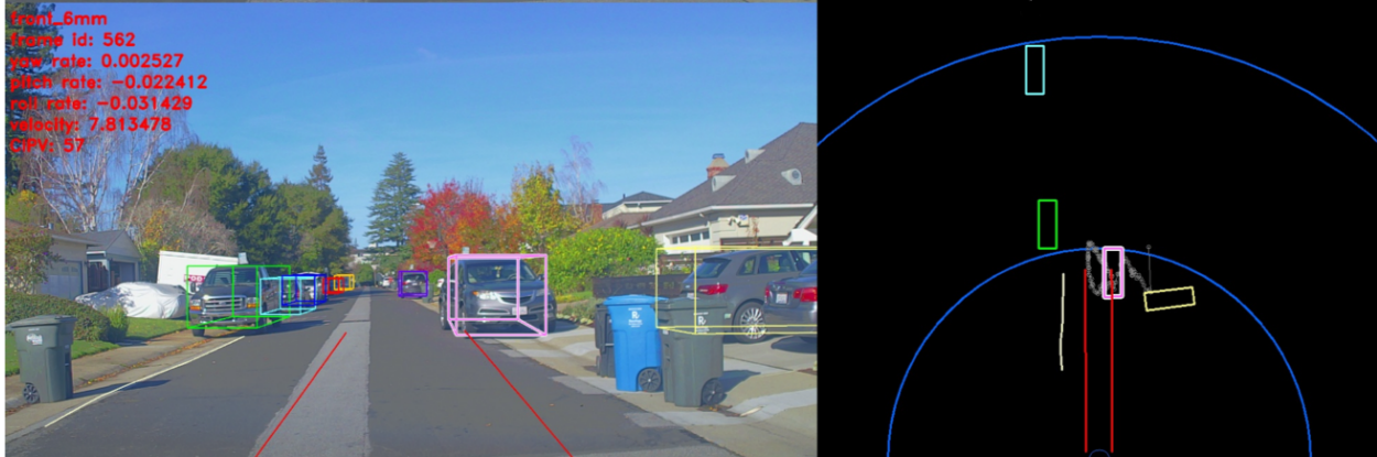
Fig. 4: Illustrative example detected objects using Apollo. The execution time depends on the detected object number and their individual predicted class.
