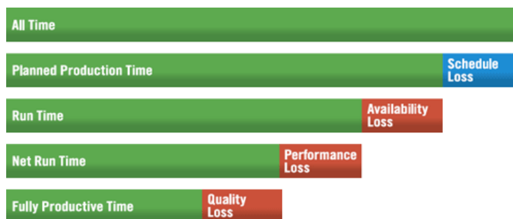
Figure 1 Effect of availability, performance and quality losses to the Planned Production Time. Source: [4]
