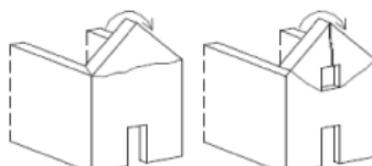
(b) Overturning of the upper part of the façade
