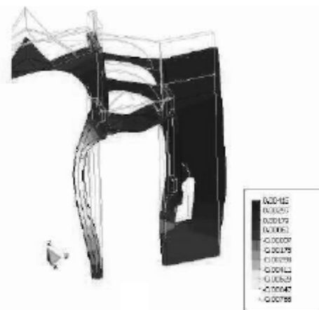
Deformed shape of the typical bay corresponding to the instantaneous gravity load obtained by (Clemente (2006)).
