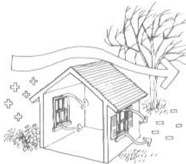
Figure 3.5 Ventilation by air
