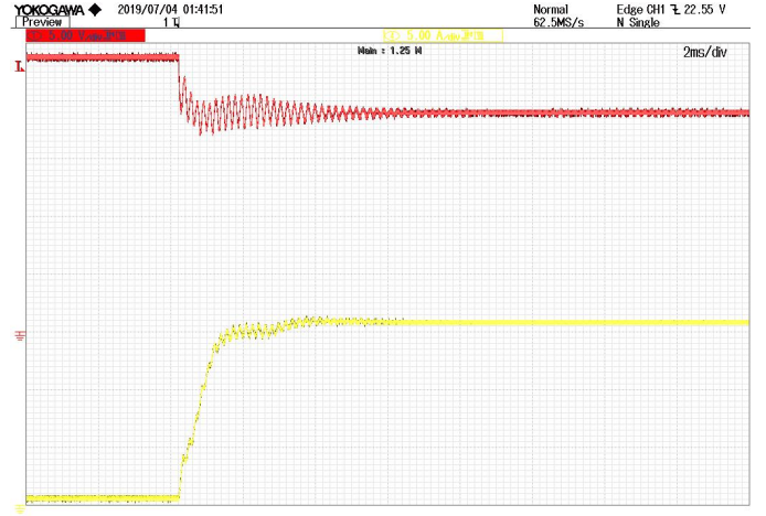
Fig. 15. System response to a step from P = 10 W to P = 300 W with the controlled shunt damper. Red curve (above) corresponds to the voltage x_2 (5 V/div) and yellow curve (below) to the current x_1 (5 A/div). Time scale is 2 ms/div.
