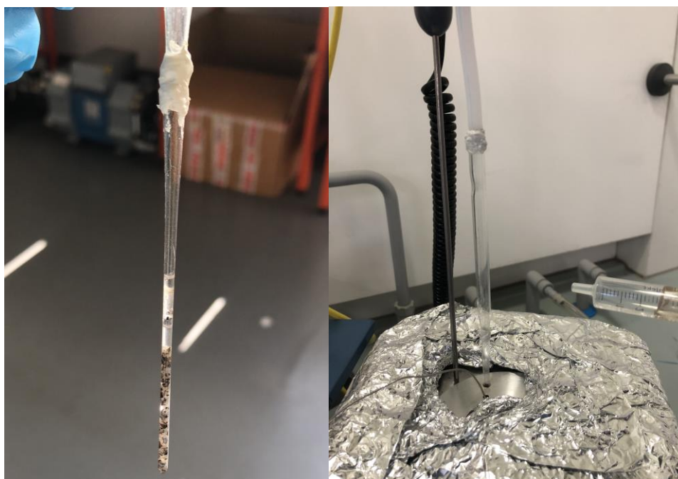
Fig. 3.16. On the left, capillary attached to the bottom part of a cut pipette with epoxy. On the right, compressed air is directed to the pipette in the new setup.
