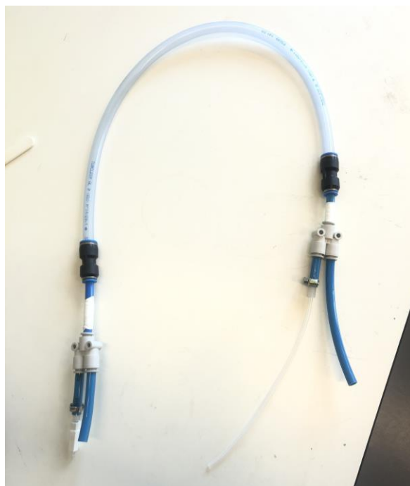
Fig. 3.14. Handmade co-current flow heat exchanger.
