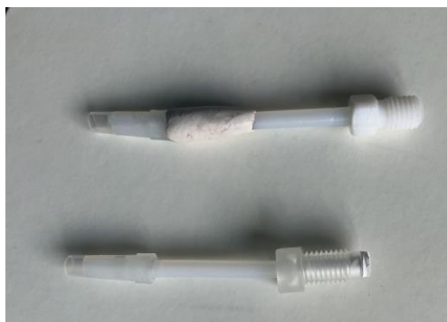
Fig. 3.12. Handmade connection for the PTFE tubing and the capillary.
