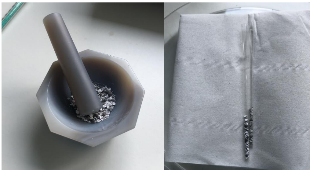
Fig. 3.11. Grounded \text{Al}_2\text{O}_3 catalyst was achieved with an agate mortar and then introduced in the capillary.
