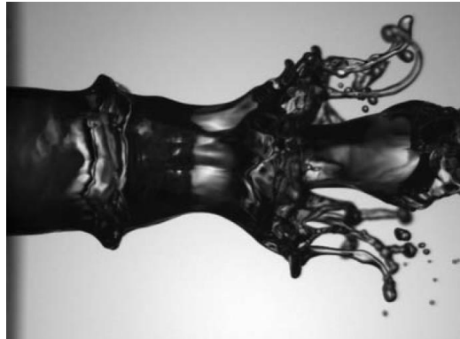
Figure 9 13 Breakup regime of a slow dense liquid jet by a fast light coaxial stream for higher gas velocity
