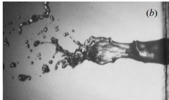
Figure 10 15 Instantaneous flow visualization of the brak-up of a liquid jet by an annular air jet.
