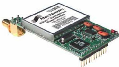
**Fig.2.20.**Xstream OEM RF module
