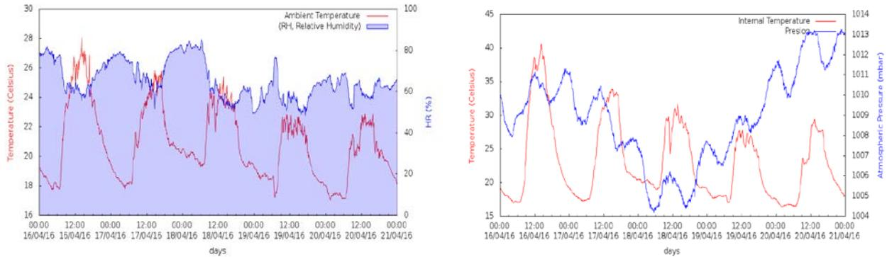
Figure 3 Data plot of a system test during a period of one week. On the left humidity with its own temperature sensor, on the right atmospheric pressure with its own temperature sensor
