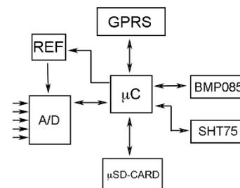
Figure 1. Schematic of the datalogger
