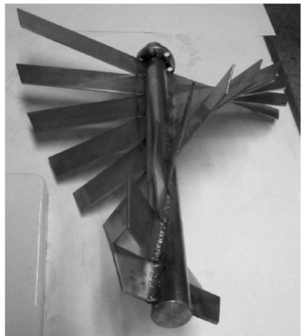
Fig. 2. Experimental stirrer used in pilot tests.
