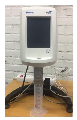
Figure 3.3: DV2T Brookfield LV viscometer.
