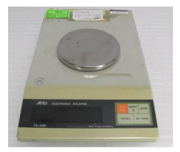
Figure 3.1: Electronic balance, FX-300 AND, used for blend preparation and dentisty determination.
