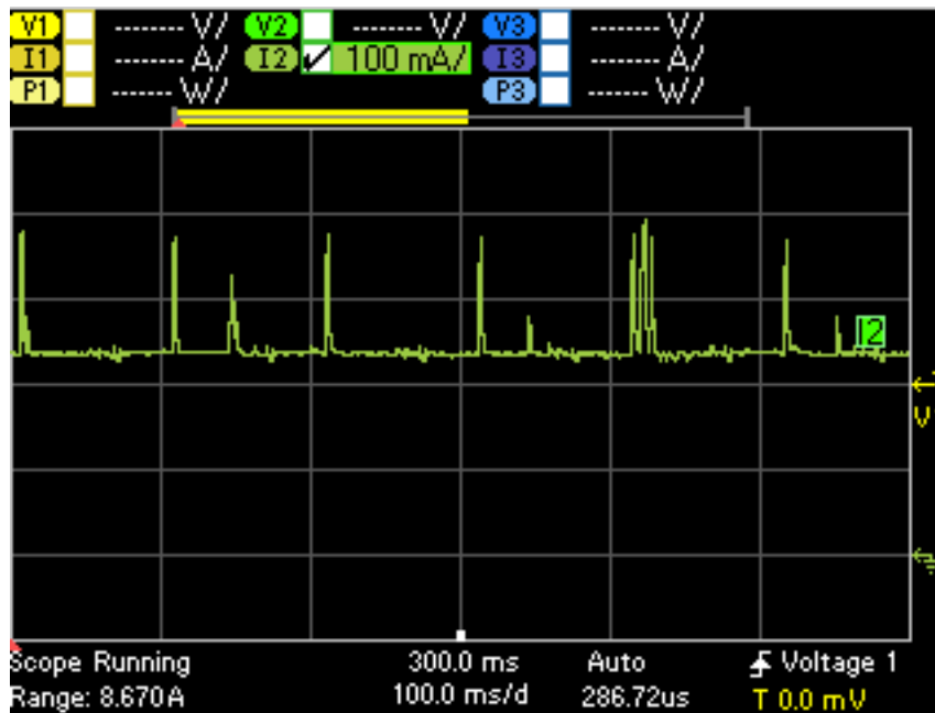
Figure 24. AP ON and one user connected via Wi-Fi – current consumption
