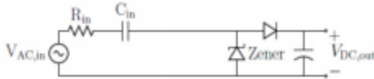
Figure 46. Capacitive power supply
