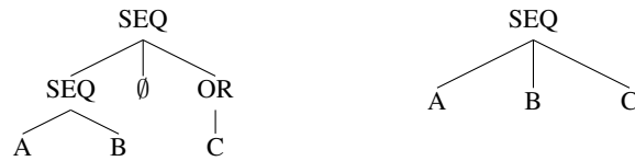
Fig. 3. Two process trees modeling exactly the same behaviour. The left model is reducible, and the right model is its irreducible representation. The silent transition \emptyset is removed because it is not part of an OR structure. The OR elementary node does not provide behavioural information.
