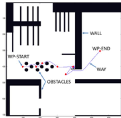
5. The simulation result of navigation and of the obstacle detection and avoidance.
