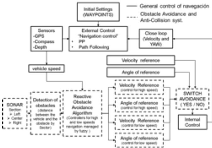
1. Block diagram of the control system of navigation and avoidance of AUV Guanay II
