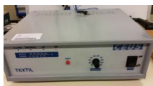
Figure 5. Left: external vibrations generator. Right: burnishing tool attached to milling machine.
