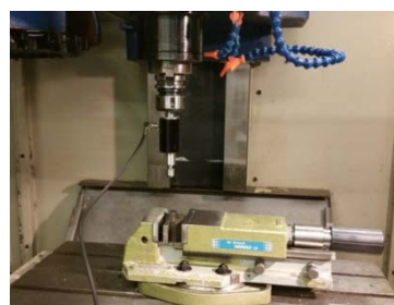
Figure 5. Left: external vibrations generator. Right: burnishing tool attached to milling machine.
