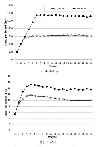
Fig. 1: Performance scalability on architectures with 6 logical cores
