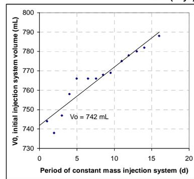
Fitting the constant mass system for different periods allowed estimating the initial injection volume of air (piston and air lines), as shown in the figure on the left.
