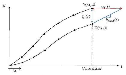
Fig. 3. Estimation of the current accumulation  $Q_i(t)$
