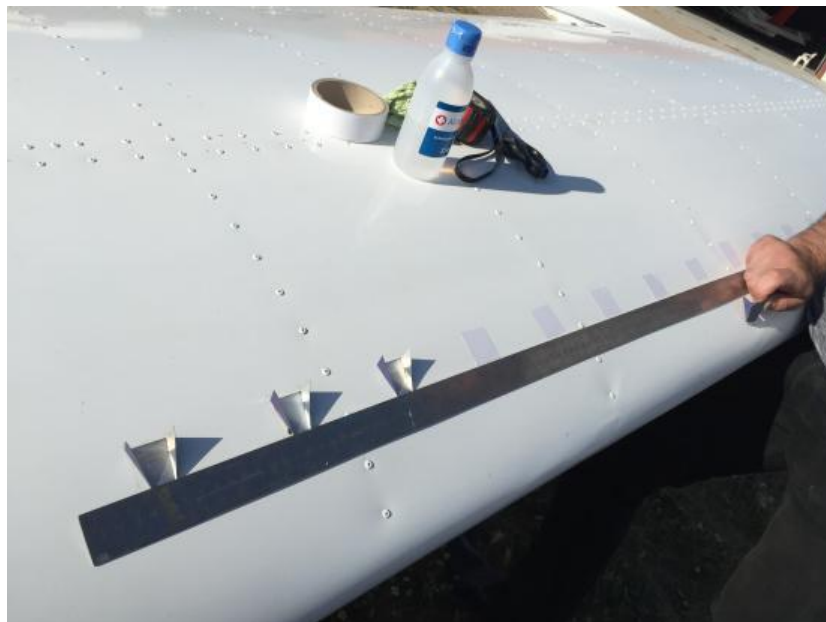
Figure 11: Process of cleaning the leading edge and sticking the VGs to the aircraft wing
