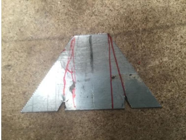
Figure 8: Aluminum base piece to create the VGs
