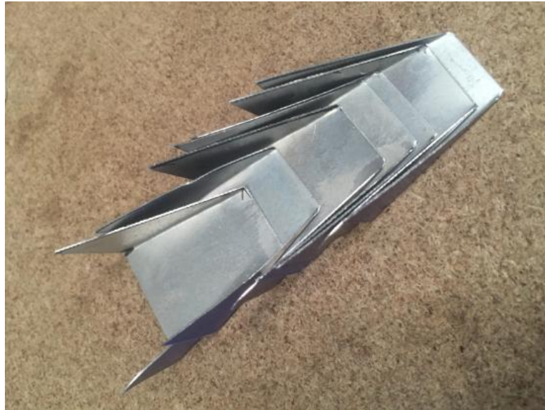
Figure 10: Various VGs constructed ready to be mounted on the wing
