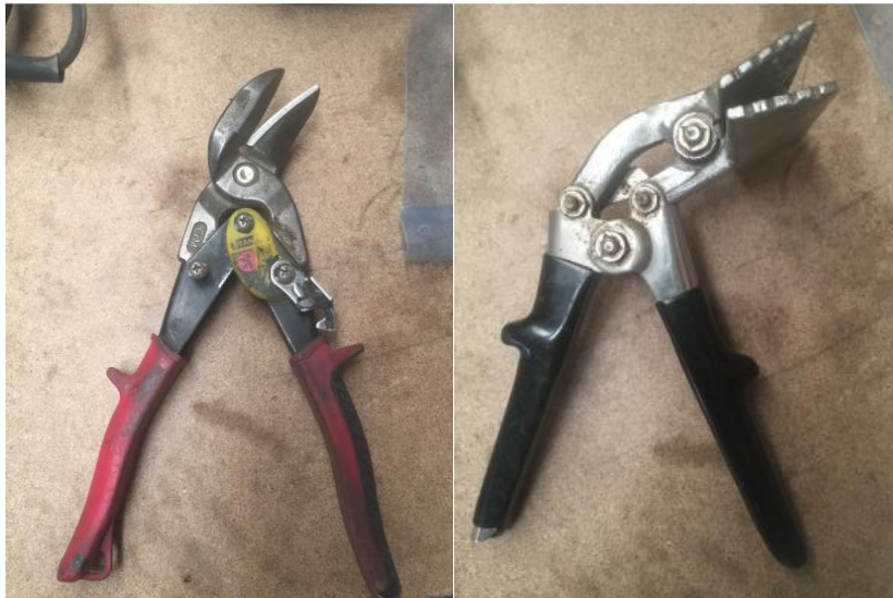
Figure 9: Tools used to cut and bend the aluminum piece
