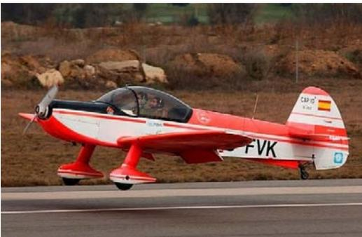
Fig. 1: Mudry CAP10B aerobatic aircraft used for educational parabolic flight campaigns. (Photo: Barcelona Flight School)
