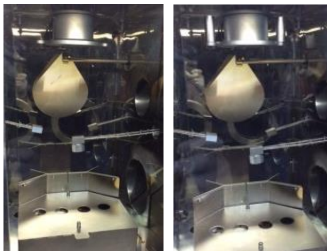
Figure 3.12. Evaporator's cavity with (right) and without (left) rotation set ups. The setup for cooling does not allow for rotation because the holder is fixed by two magnets.
