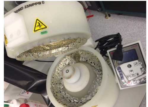
Figure 3.4. Spin-coater WS-650MZ-23NPP, Laurell Technologies. This one was used inside the fume hood to deposit the ZnO layer.
