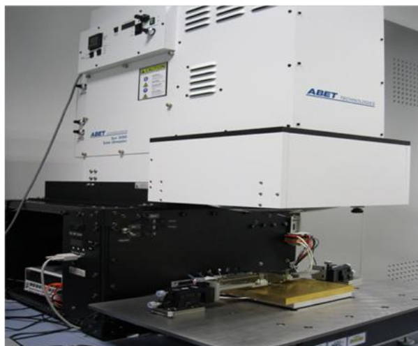
Figure 31: Solar simulator class AAA from ABET technologies. Temperature can be kept at 25 °C for standard measurements.
