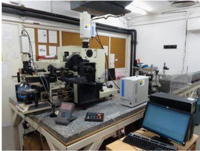
Figure 30: T64000 Horiba-Jobin Yvon. Pre-resonant conditions for ZnSe detection are achieved with a blue excitation laser wavelength.
