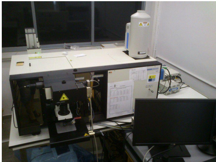
Figure 29: LabRam HR800-UV Horiba-Jobin Yvon suitable for Raman mapping measurements.
