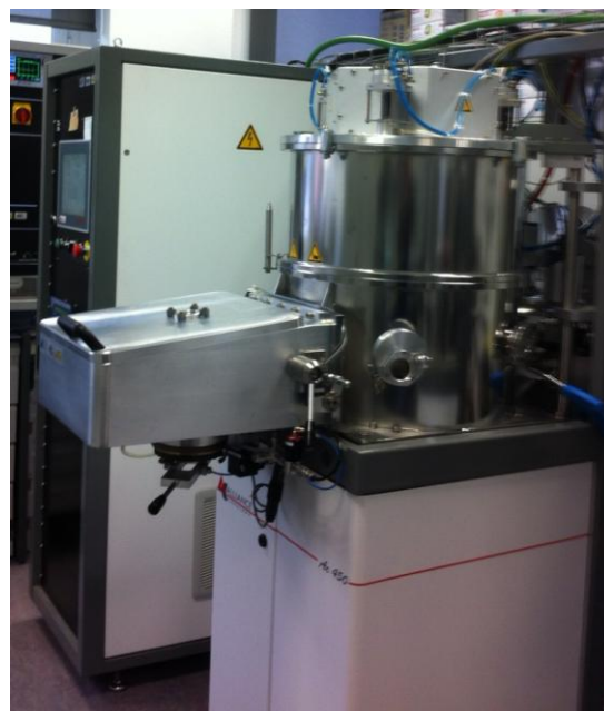
Figure 25: AC 450 Alliance concept DC sputtering system. Three cathodes are on top of the circular deposition chamber.
