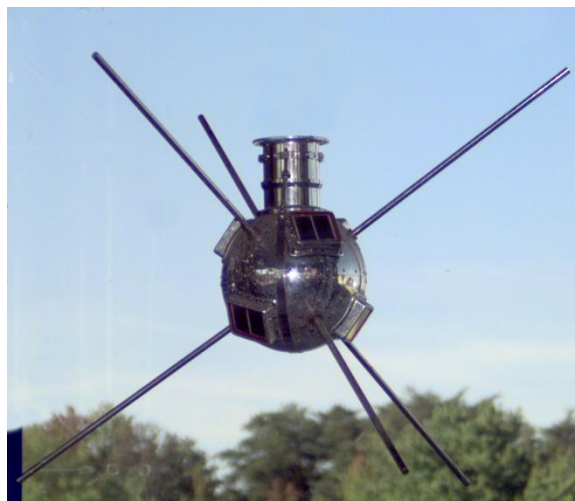
Figure 2: Source: NSSDC-NASA COSPAR ID: 1958-002B. Satellite Vanguard I with six square (roughly 5 cm on a side) solar cells mounted on its body.
