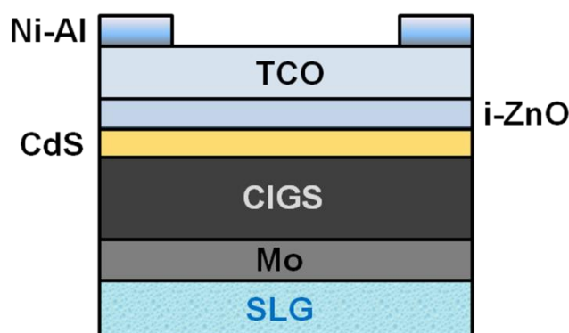
Figure 12: Cross sectional view of a CIGS thin film solar cell on SLG substrate.
