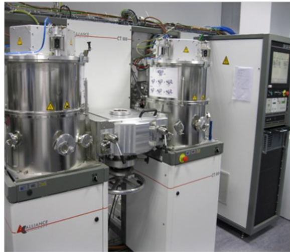
Figure 28: CT100 Alliance concepts for DC-pulsed magnetron sputtering of the window layers.
