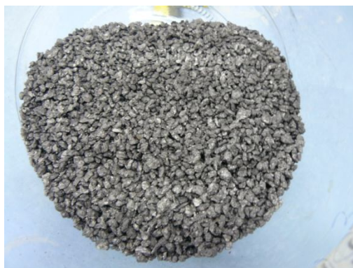
Figure 3.4 Picture of the granular graphite used as anode and cathode in the MEC BC1 and BC2.
