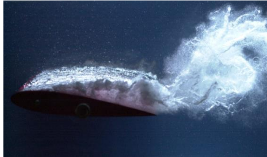
Figure 42. Cavitation in a hydrofoil (13) .
