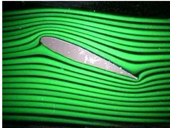
Figure 5. Streamlines around a hydrofoil.
