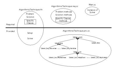
Fig. 1. Architecture of a MALLBA skeleton
