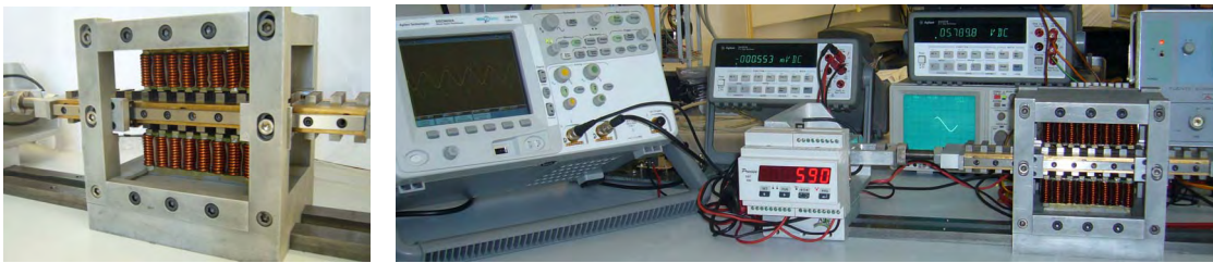
Fig. 9: View of LSRM prototype and experimental setup
