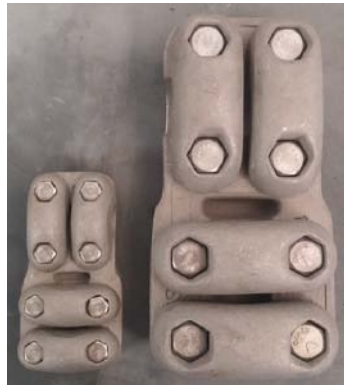
Figure 1: HTLS connector's reduced-scale (left) and original-scale (right) used to perform the tests described in the following lines
