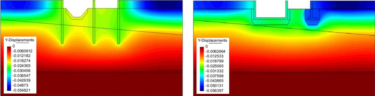
**Figure 3:** Vertical displacement for the plastic analysis.
