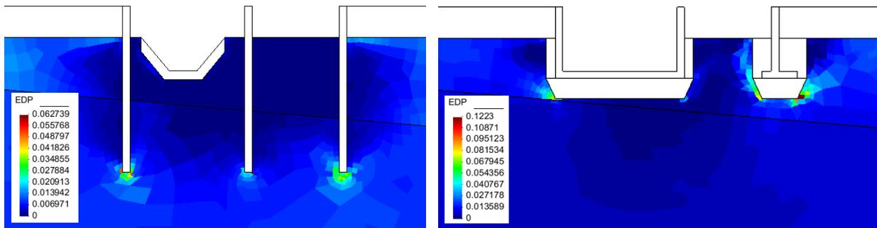
Figure 4: Shear plastic deformation due to the overloading.
