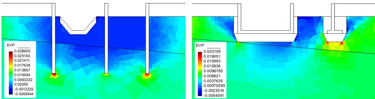
Figure 5: Volumetric Plastic deformation due to the overloading.
