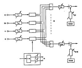
Fig.9: Simplified block diagram of the digital beamforming ASIC
