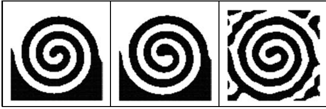
Fig. 4. Generalization obtained by SVM-Light (left), BPW with gaussian functions (center) and BPW with sine functions (right) for the Two Spirals problem. The results for BPW are the mean over 10 runs.
