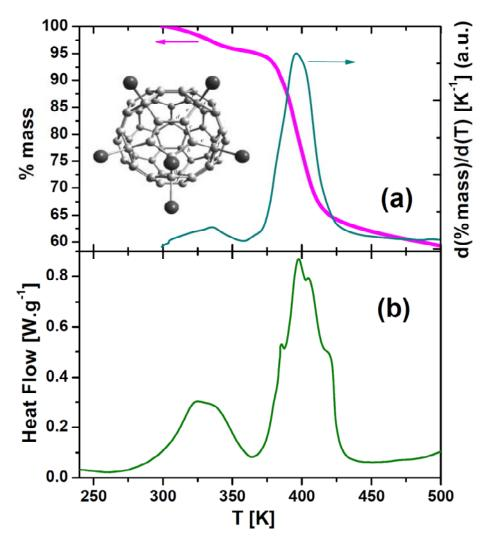
**Fig. 1**. TGA (a) and DSC (b) curves measured on the as-synthesized  $C_{60}Br_6$  powder upon heating. In (a), the thin line is the first derivative of the percent mass loss (thick line), and the molecular structure of  $C_{60}Br_6$  is shown as inset.
