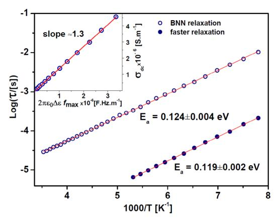
**Fig. 4.** Arrhenius plot of the characteristic times  $\tau$  of both dielectric loss features in C<sub>60</sub>Br<sub>6</sub> (markers), and corresponding Arrhenius fits (continuous lines). Inset: plot of  $\sigma_{dc}$  versus the quantity  $2\pi\epsilon_0\Delta\epsilon/\tau$  calculated for the most prominent dielectric loss. The continuous line is a linear fit to verify the validity of the BNN relationship below 230 K (see the text).
