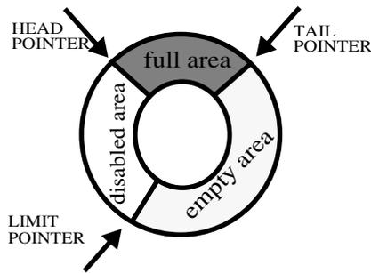
**Figure 7:** The instruction queue with resizing capabilities.
