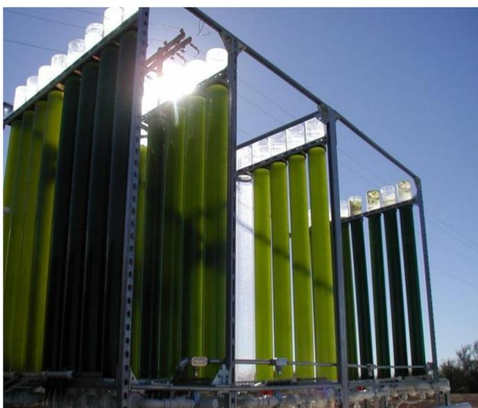
Figura 6: Fotobiorreactor de columna. Fuente: <http://www.nanovoltaics.com/content/algae-photobioreactors>
