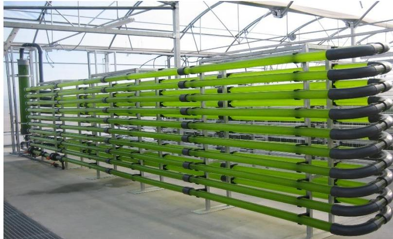
Figura 7: Fotobiorreactor tubular vertical. Fuente: [www.algaenergy.es](http://www.algaenergy.es)
