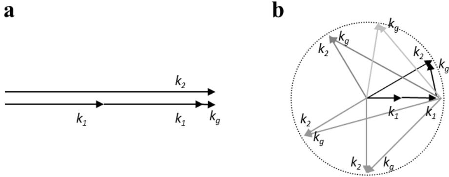
**Figure 1.5:** Schematic of the phase-matching relation between  $k_1$ ,  $k_2$ , and  $k_g$  in the case of SHG in disordered media. (a) Collinear SHG. (b) Non-collinear SHG.
