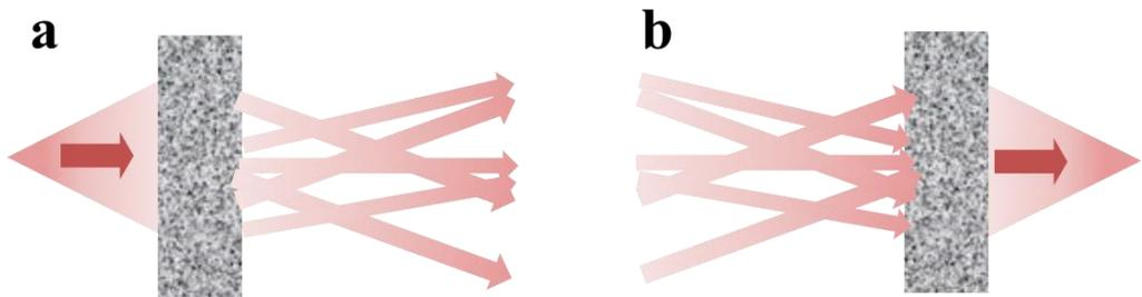
**Figure 1.2:** Schematic of (a) light scattering through a diffusive material and (b) light focused after one diffusive material under a wave-front shaped incident beam.
