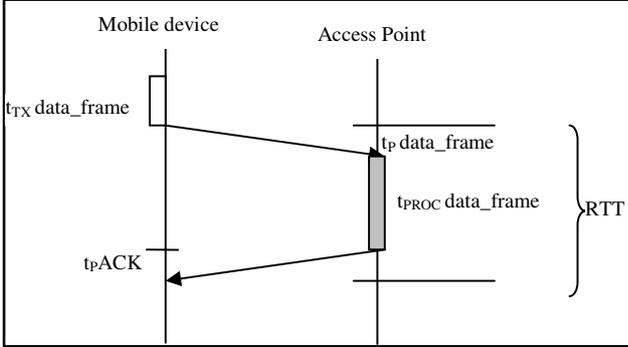
Figure 1. *RTT* measurement using IEEE 802.11 data/ACK frames
