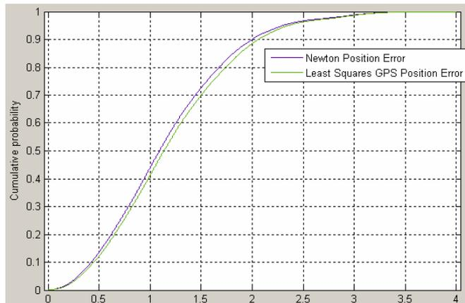
Figure 6. CDFs' positioning error (MT inside the triangle)
