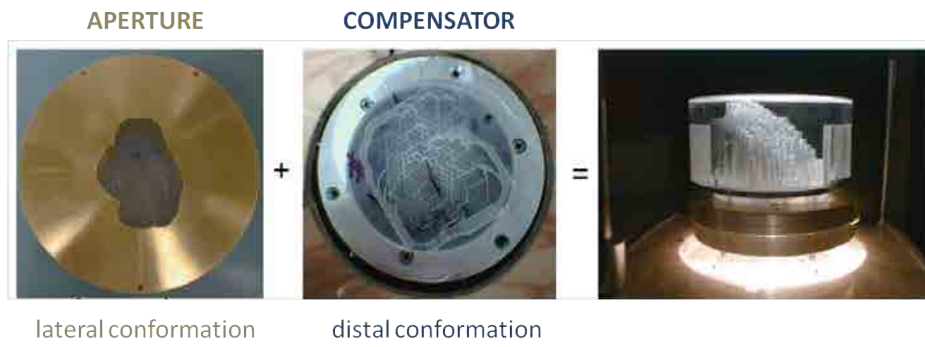
Figure 1.5: Patient-specific devices for dose conformation to the tumor in passively-scattered proton therapy fields.
