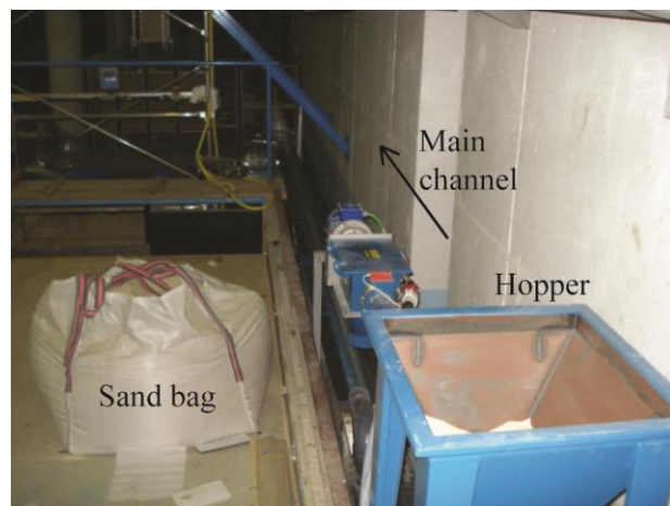
Figure 3.2. Arquimedes screw hopper used to feed the model with sediment. The model inlet is under the hopper engine and follows a direction parallel to the
