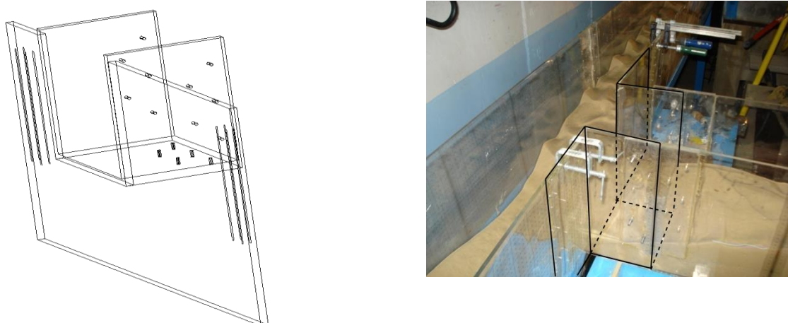
Figure 1.11. Scheme and photograph of the bifurcation piece. The piece extends deeper than the main channel to allow its raising to establish a bed discordance between both branches.
