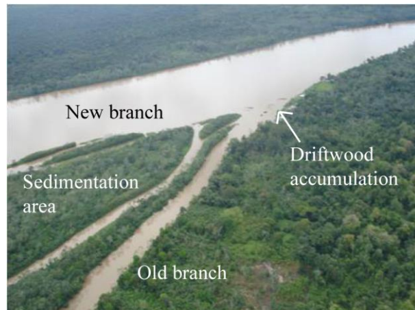
Figure 1.6. Close aerial view of the present situation of the Patia River bifurcation.
