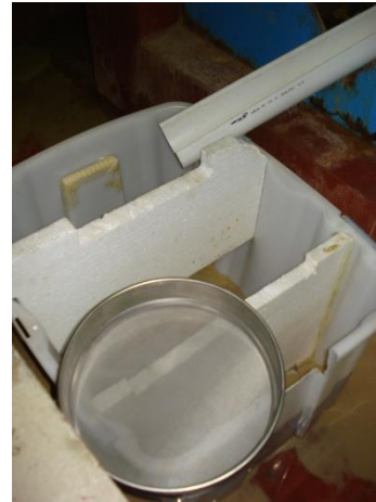
Figure 3.4. Outlet of the lateral branch: settling tank and sieve for solid discharge measurements
