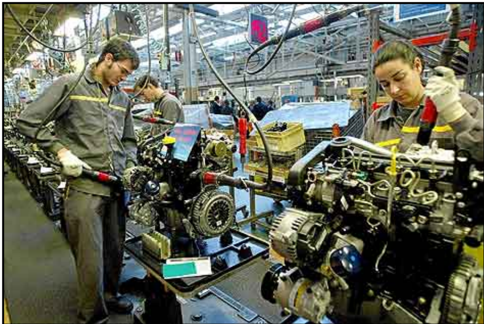
Figure 46- Continuous flow organization of the production lines at Valladolid engines. (Source: elmundo, 2012)
