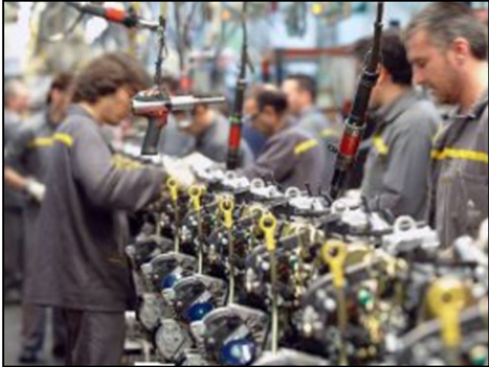
Figure 45- Continuous flow organization of the production lines at Valladolid engines. (Source: Automocionqualiauto, 2012)
