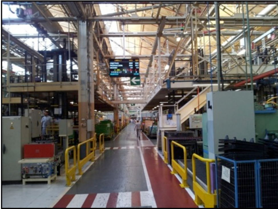
Figure 47- Plant photo during the visit at Valladolid Engines. It can be observed the continuous flow organization of the production lines (Source: plant photo during the visit).
