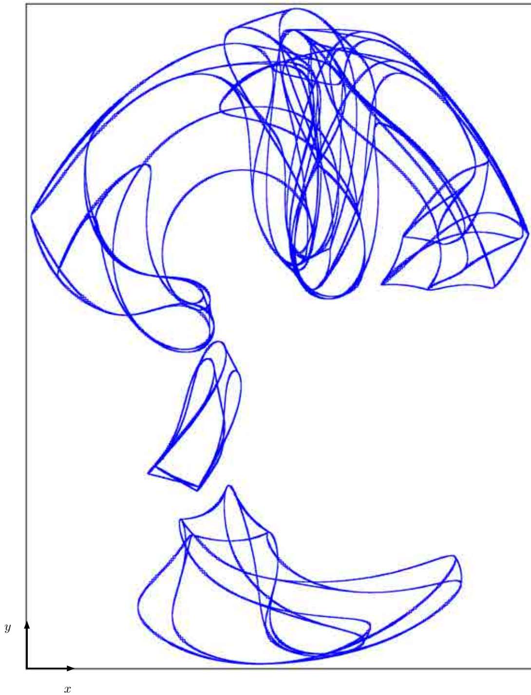
Figure 4.8: Box approximation of the set \pi_u(\mathcal{S}) corresponding to the reachable workspace of the linkage in Fig. 4.7.
