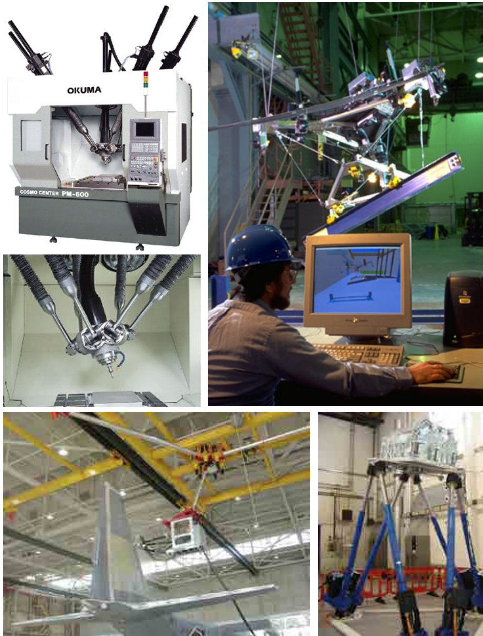
Figure 6.2: From left to right and top to bottom: The Okuma PM-600 machining center (top), and a close-up of the hexapod platform holding the tools (bottom) [124]; a worker programming and monitoring the TETRA RoboCrane from the NIST [125], used to pick up and place a steel beam in a stanchion; a cable-driven hexapod for aircraft building and maintenance [125]; and a swell simulator [126].
