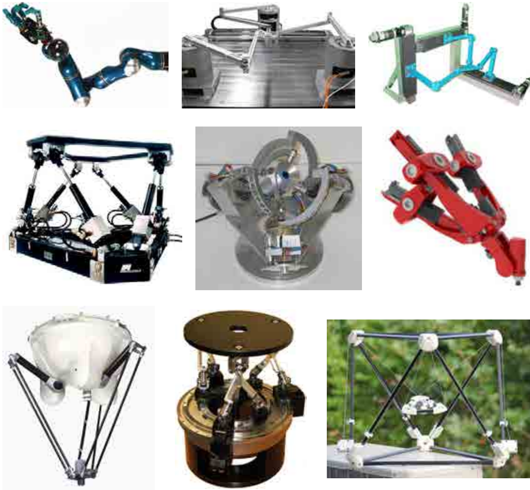
Figure 1.3: Left to right and top to bottom: The DLR LWR arm and hand [36], a 3(P)RRR planar reconfigurable manipulator [37], the tripteron mechanism [38], a commercial Stewart platform [39], a spherical parallel manipulator for the rapid orientation of a camera [40], the exechon X700 parallel kinematics machine [41], the Kawasaki Delta YF03N manipulator [42], the rotary hexapod MicARH for micropositioning [43], and the IRI hexacrane [44].
