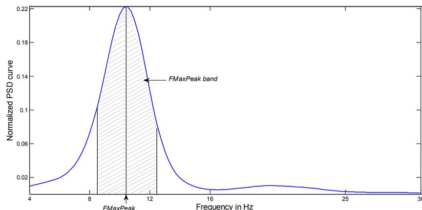
Figure 34 Example of a power spectral density curve for arousal signal. After the maximum peak value (FMaxPeak) of the spectrum is calculated (s7), then we create a band around that peak (FMaxPeak  $\pm$  2Hz) and we are able to calculate four other features: s8) the ratio of FMaxPeak band over the total power spectrum; s9) skewness and s10) kurtosis of the FMaxPeak band.
