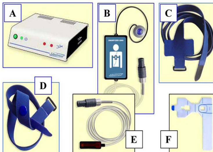
Figure 8 Snoryzer Uno equipment: A - acquisition system, B - tracheal microphone, C - chest band, D - microphone wrapping band, E - pulse oximeter sensor, F - adhesive for fixation of the pulse oximeter sensor (from SIBEL S.A.).
