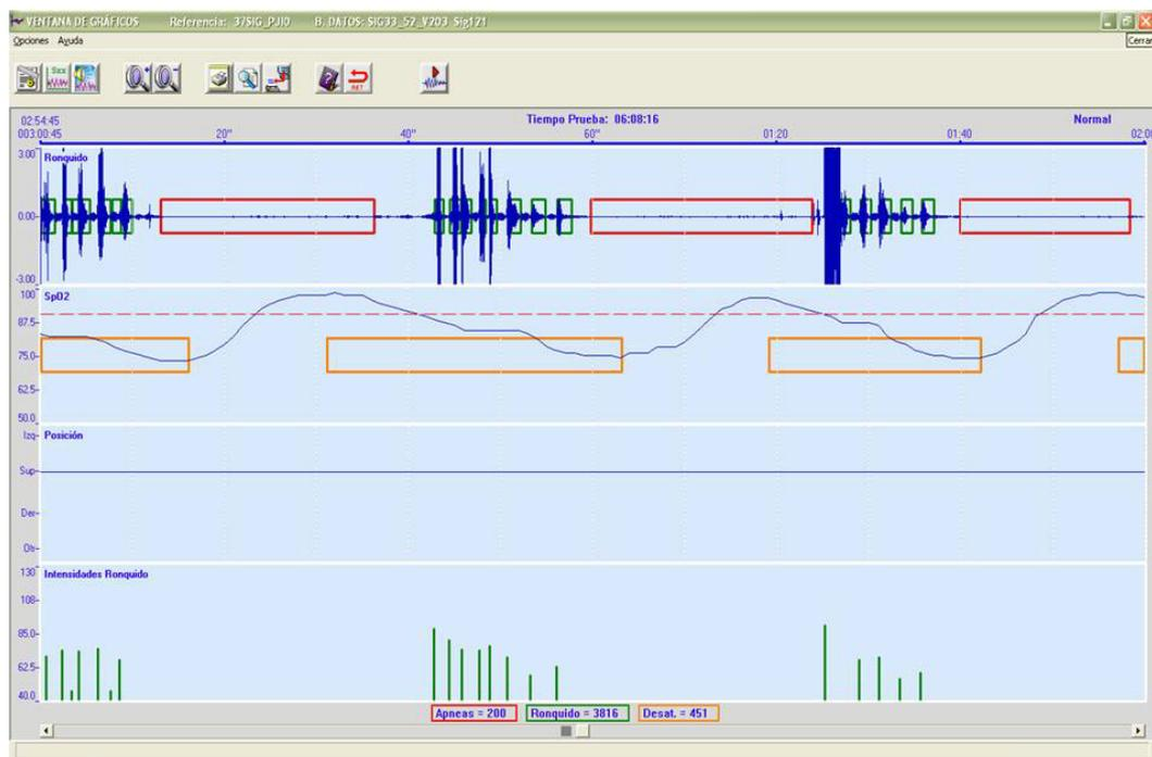
Figure 9 Example of a 2 minutes registration with Snoryzer Uno. The superior panel shows the respiratory sound signal where one can observe the labeled snores as well as 3 apnea episodes. The second panel shows the oximetry signal where the desaturations indicate that an apnea has just occurred. The third panel shows the sleeping position and the last panel shows the detected snoring episodes (the height of the bar indicates the snore episode intensity).
