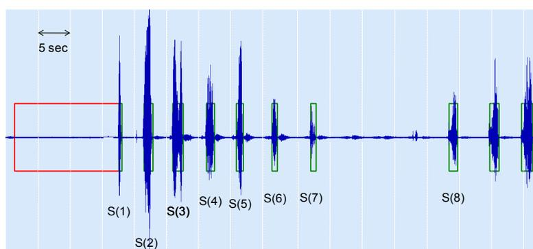
Figure 20 Excerpt of a snoring sound signal. The dashed line box corresponds to an apnea episode and the solid line boxes correspond to snore episodes. S(1) is a post-apneic non-regular snore. All S(2) - S(7) snores are regular snores. S(8) is a *normal* non-regular snore.
