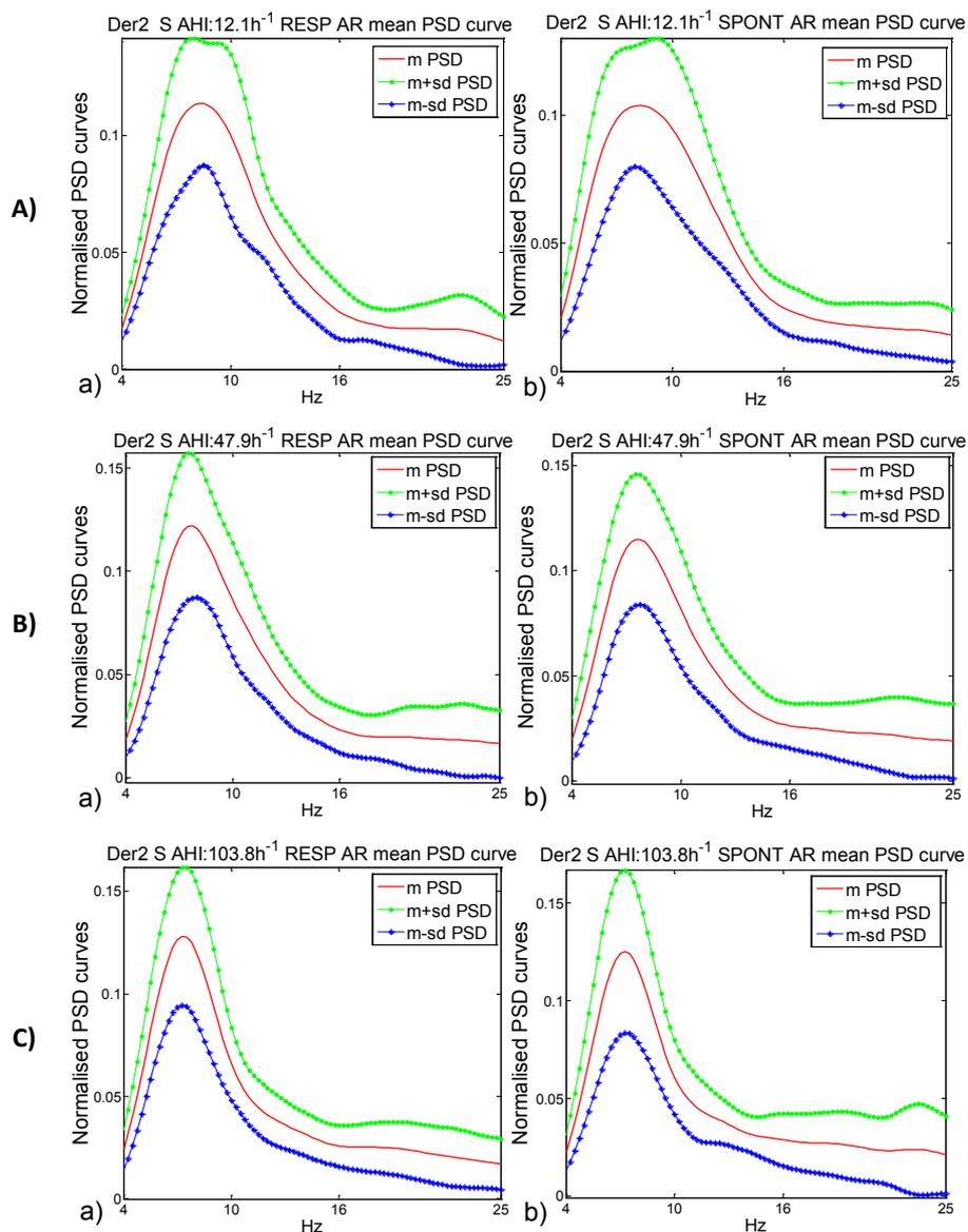
Figure 44 For derivation C4A1 (Der2). a) respiratory and b) spontaneous arousals mean and  $m \pm sd$  PSD curves for a A) mild SAHS subject ( $12.1h^{-1}$ ), a B) severe SAHS subject ( $47.9h^{-1}$ ) and a very severe SAHS subject ( $103.8h^{-1}$ ). The mean PSD curves were computed out of a total of Aa) 16 respiratory arousals and Ab) 64 spontaneous arousals; Ba) 65 resp and Bb) 44 spont; Ca) 106 resp and Cb) 37 spont.
