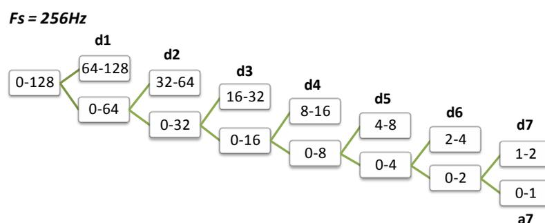
Figure 33 Wavetree for  $f_s=256\text{Hz}$ , with all decomposed components. Our vector of features  $M_x$  is composed of: m1) detail coefficient d3, m2) detail coefficient d4; m3) detail coefficient d5; m4) detail coefficient d6 and m5) detail coefficient d7.
