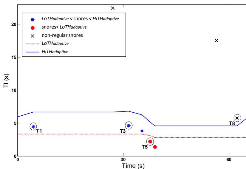
Figure 15 Performance of  $LoTH_{adaptive}$  and  $HiTH_{adaptive}$  on the time interval between successive snores  $TI(i)$  of the short segment signal shown in Figure 14.
