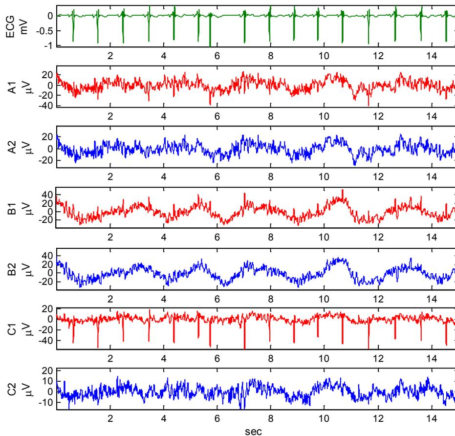
Figure 30 Short 15 second segment of ECG and EEG signals. A1, B1 and C1 correspond to the EEG contaminated tracings, C3A2, C4A1 and O1A2, respectively. A2, B2 and C2 correspond to the clean EEG tracings, C3A2, C4A1 and O1A2, respectively.
