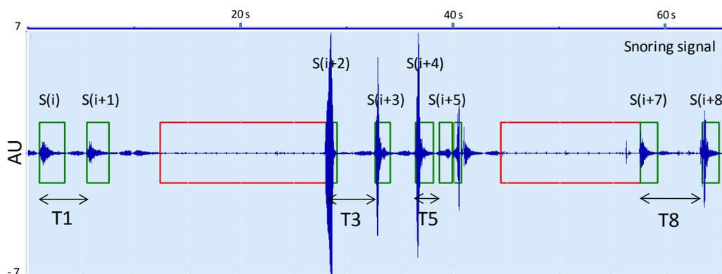
Figure 14 Example of an excerpt of a snoring sound signal from a subject in our database. The small boxes correspond to snore episodes. The two wider boxes correspond to two apnea episodes. T1, T3, T5 and T8 are the time intervals between the snores:  $S(i)$  and  $S(i+1)$ ,  $S(i+2)$  and  $S(i+3)$ ,  $S(i+4)$  and  $S(i+5)$ ,  $S(i+7)$  and  $S(i+8)$ , respectively.
