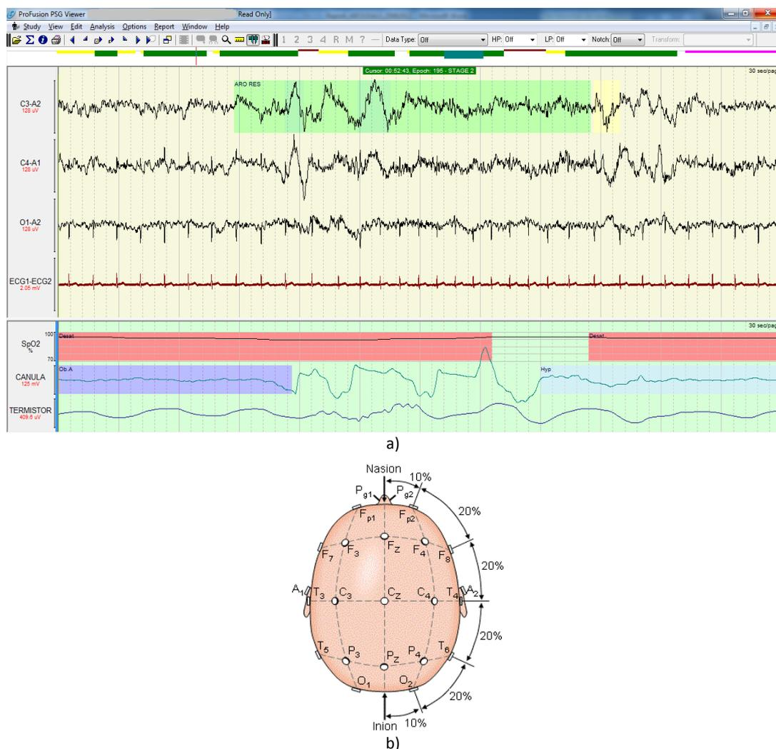
Figure 28 a) Profusion PSG 2 software printscreen with a respiratory arousal event marked on the C3A2 tracing and corresponding obstructive apnea marked on the cannula signal. b) Electrode placing positions for EEG acquisition.
