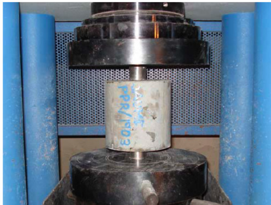
Figure 2.6: Scheme of the double punch test (Guàrdia (2007))
