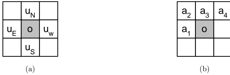
Figure 3.11: (a) Support and notation for the 4-tap ULS on the quincunx grid. (b) Typical geometry of a 2-D auto-regressive neighborhood. Four pixels are used for generating the pixel at site ‘o’.
