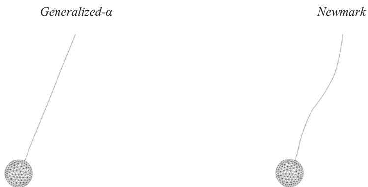
Figure 3.31 Deformed cable at time 2.18 s.
