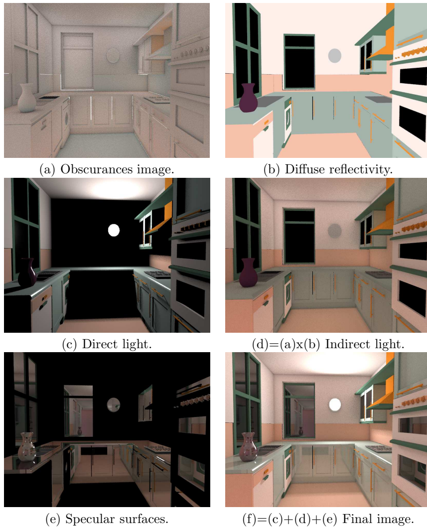
Figure 6.1: These six images show the contribution that each kind of ray of our rendering algorithm give to the final image and how it is computed. The first image (a) shows our main contribution: the obscuration. The second (b) image shows the diffuse color of each object in the scene. By multiplying both images we get indirect light image (d). Direct light is shown in (c). Adding the contribution of the specular surfaces (e) to (c) and (d) we get the final image (f). All the images of the kitchen scene shown here have a resolution of 800x600 pixels.
