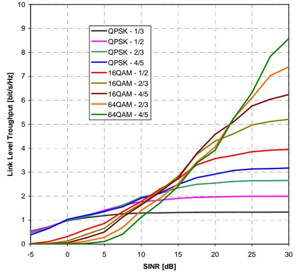
Fig. 8 E-UTRA DL 2x2 MIMO MMSE link level throughput with H-ARQ in multipath EPA channel 3km/h and medium antenna correlation
