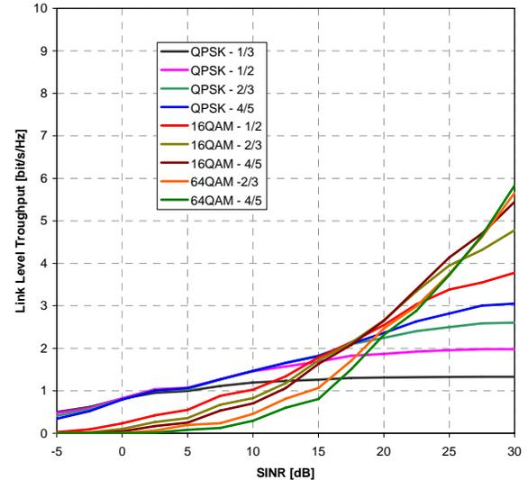
Fig. 9 E-UTRA DL 2x2 MIMO MMSE link level throughput with H-ARQ in multipath EPA channel 3km/h and high antenna correlation
