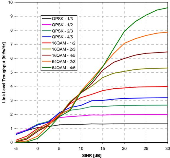
Fig. 7 E-UTRA DL 2x2 MIMO MMSE link level throughput with H-ARQ in multipath EPA channel 3km/h and low antenna correlation
