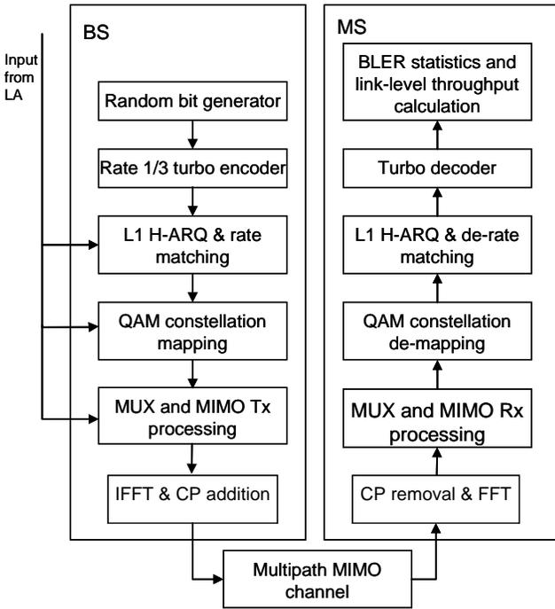
Fig. 1 Block diagram of one layer of the E-UTRA DL link level simulator
