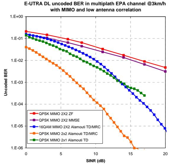
Fig. 5. Uncoded BER vs. mean SINR for different modulations and MIMO processing in EPA multipath channel @ 3km/h
