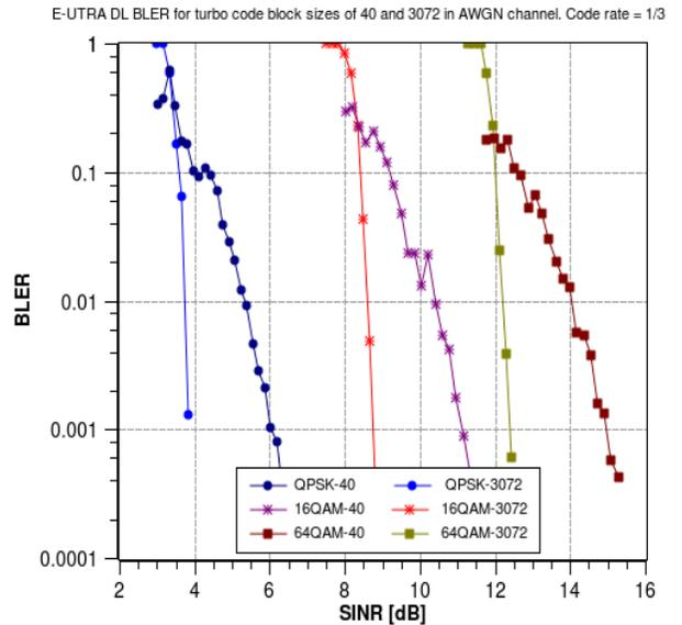
Fig. 2. BLER for two different code block sizes in AWGN channel
