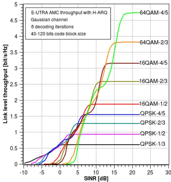
Fig. 4. E-UTRA DL AMC link level throughput with H-ARQ in Gaussian channel (Code block size: 40-120 bits)
